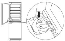
Place the lower door bearing with the bearing pivot in the lower left of the freezer compartment door and fasten.
